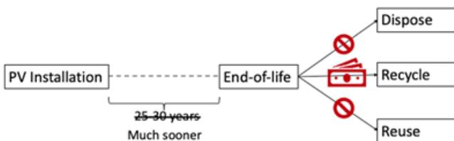
Figure 3. With early replacement, the recycling route becomes a huge bottleneck and is no longer a cost-efficient end-of-life option
